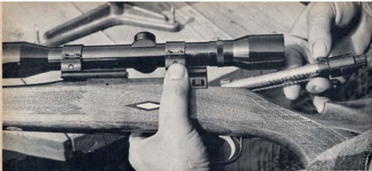
Bolt release for Sako action is located just behind shooter's thumb. Action has fast lock-time. Note fine checkering at pistol grip, forend.
