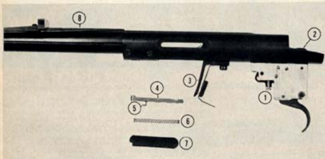
Simple bolt construction with rear locking lugs distinguishes new rimfire rifles.
